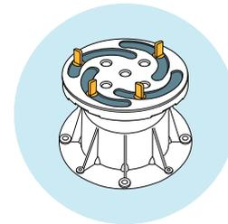
The spacer tabs snap into place and **slide into the slots**.
