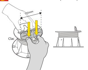
Put the joist on the support and fix with a screw
