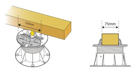
3 Screw the joist with 2 screws
