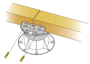
NB: The joist support to a length of 125mm and is provided with three holes for the attachment of a joist (central hole) or two sections of joists (lateral holes)
