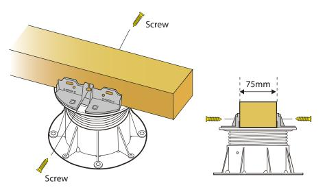
4 Put the 2 joist sections on top of the pedestal and fix them with 4 screws
