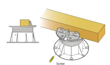
Put the two joists on the support and fix with screws
