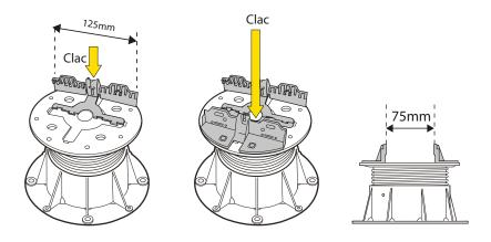
2 Put the joist of 75 mm wide on the support
