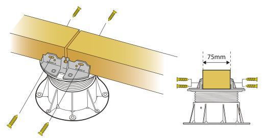
NB: The joist support to a length of 125mm and is provided with three holes for the attachment of a joist (central hole) or two sections of joists (lateral holes)
