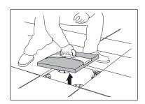
Buzon recommends using an appropriate tool to lift and set/replace the pavers. This reduces the risk of damanging the pavers or injury to the person handling them. It also helps protect the Buzon Pedestals and Spacer Tabs. Ask your Buzon Dealer or Buzon contractor installer to supply lifting tools. Various tools can be found in local hardware stores.
